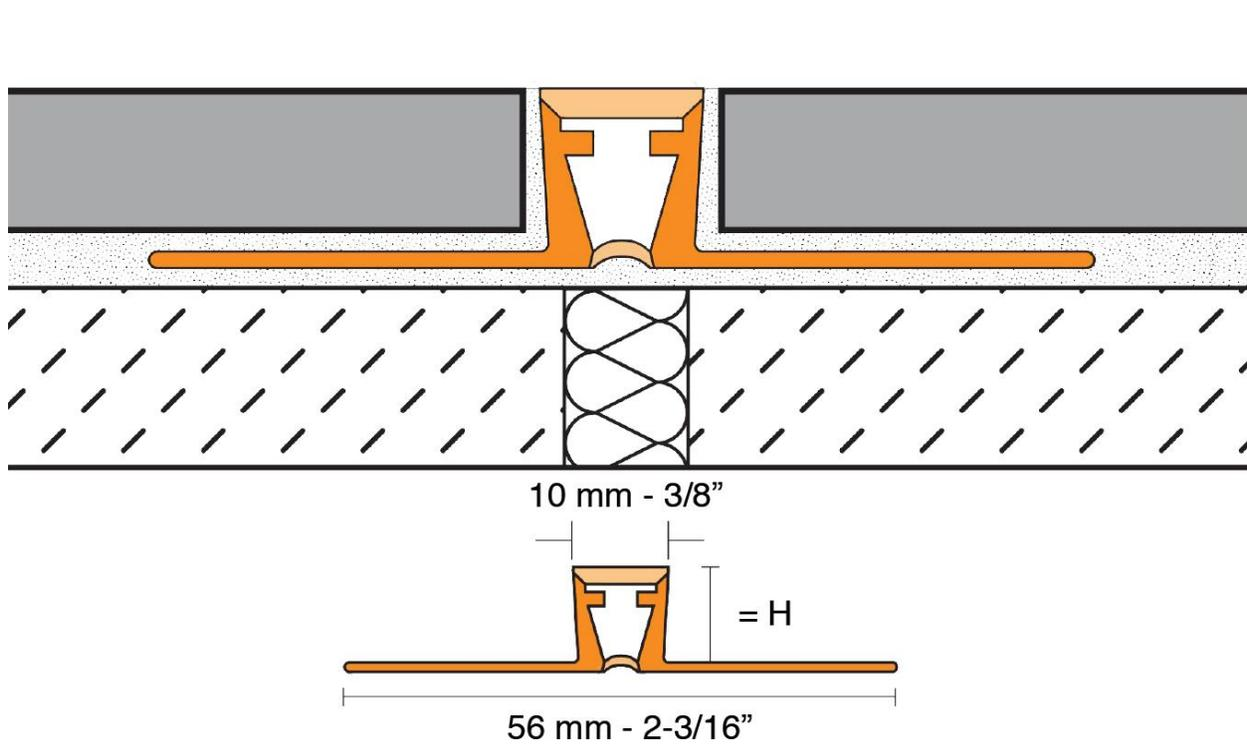
**Recommended to use as an expansion joint with Liquid Elements Crush.**
